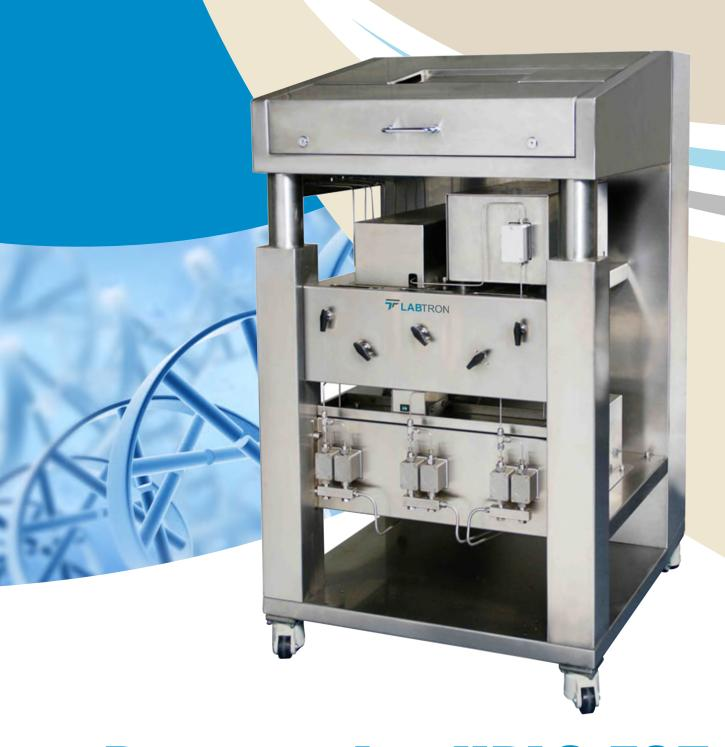
Preparative HPLC-705 is equipped with 4 pump head variation and a UV or RI detector with a wavelength range of 190 to 400 nm and 400 to 800 nm. Built in multi positioned fraction valve and controlled fractionation optimizes controlled fraction collection and solvent recycling. With a column size of  $10 \times 1000$  mm the retention, resolution and selectivity is optimized
